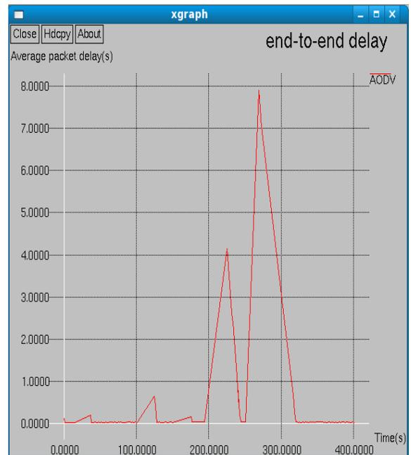
Figure.8 packet delay
