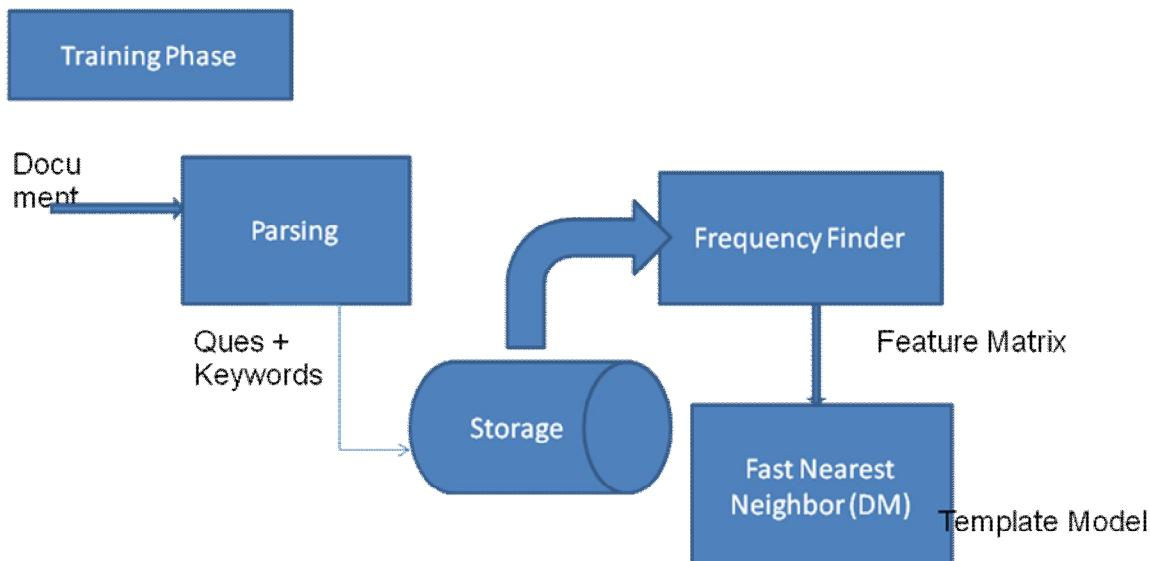
Fig:1 FNN Block Diagram phase1
