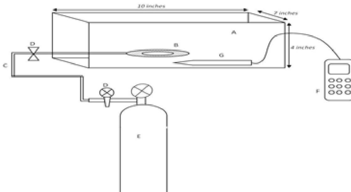
**Figure 1.** Schematic diagram illustrating the hypoxia-inducing chamber: (A) Polypropylene chamber (B) Gas diffuser (C) Pipeline for introduction of  $\text{N}_2$  gas (D) Pressure valves (E) Nitrogen cylinder (F) Dissolved oxygen (DO) meter (G) DO probe.
