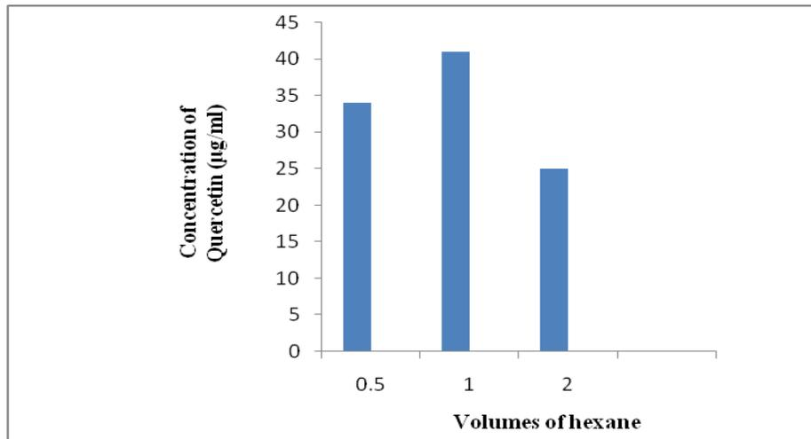
Fig. 7. Effect of different volumes of hexane on the extraction of quercetin
