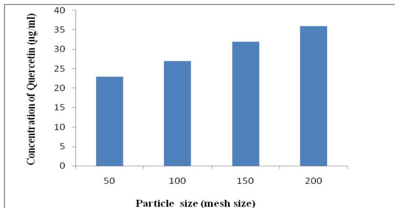
Fig. 5. Effect of different particle mesh sizes on extraction of quercetin
