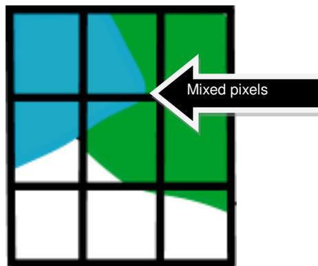
Fig 2: The mixed pixel problem. Many of the pixels in this 9 cell grid contain more than one class.
