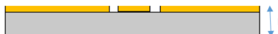
Figure 2: scheme side view of the structure illustrating the substrate and the radiating elements with total height of 2.4 mm.
