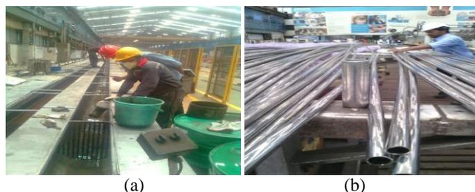
Figure 4.1(a, b): Manual Processes are carried out by manual operations; there is less automation in processes which takes more time in production. It is also possible that while manually cleaning the acid tank the workers may get harmed.
