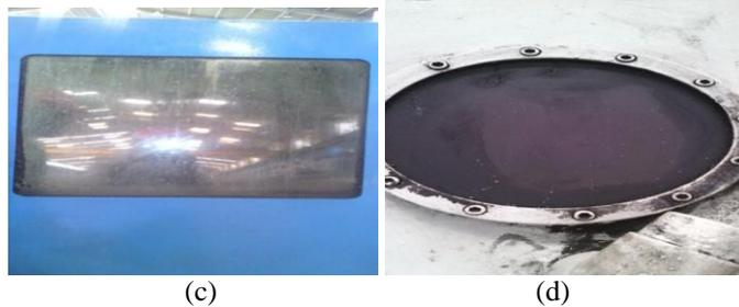
Figure 4.2(c, d): Improper visualization of machining process at end facing machine. Due to sprinkling of oil over the glass it is not possible to examine the process.
