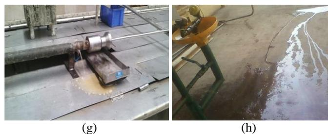
Figure 4.4(g, h): Algae/Fungus on floor due to water and oil leakage from machine makes the floor slippery. There is no provision for using the leaked oil which leads in wastage.
