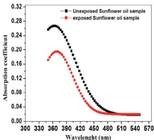
**Figure 2.** Variation of absorption coefficient as function of Wavelength of light.
