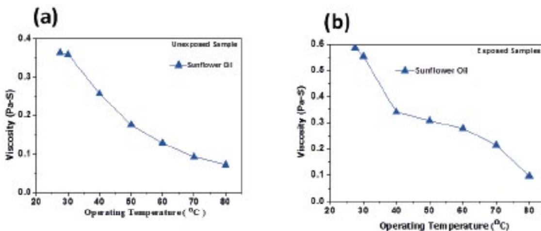
**Figure 5.** Variation of Viscosity for Sunflower oil as function of operating temperature (a) unexposed oil (b) exposed oil.
