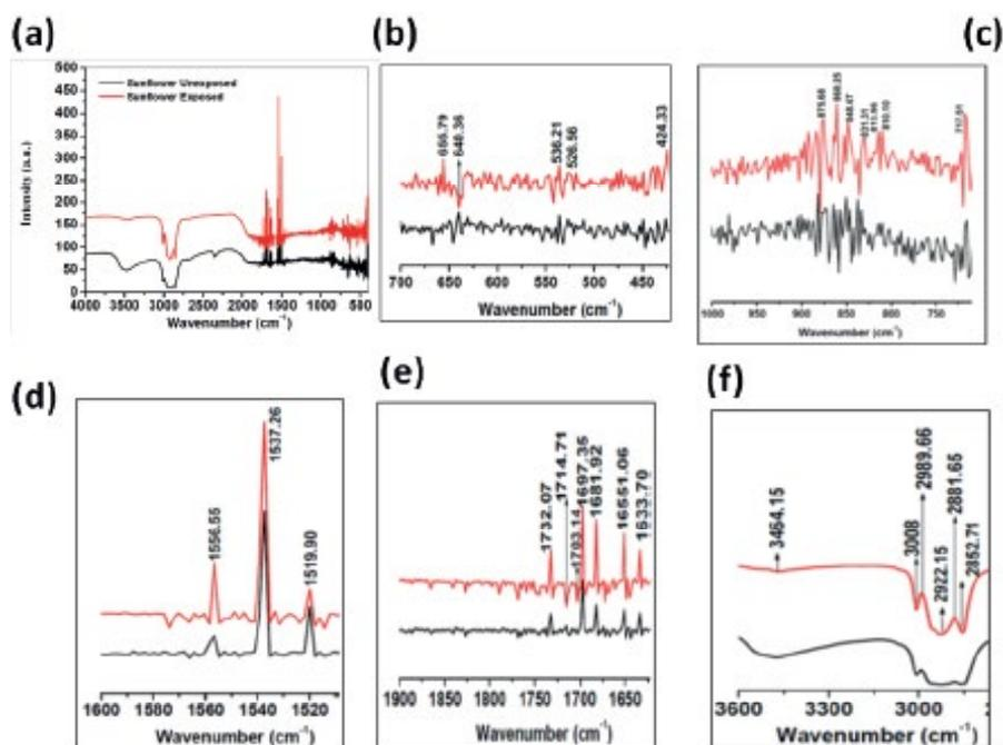
**Figure 3.** FTIR spectra of exposed and unexposed sunflower oil. (a) full Spectra, (b) 400-700  $\text{cm}^{-1}$  (c) 700-1000  $\text{cm}^{-1}$  (d) 1500-1600  $\text{cm}^{-1}$  (e) 1600-1900  $\text{cm}^{-1}$  and (f) 3000- 3600  $\text{cm}^{-1}$ .
