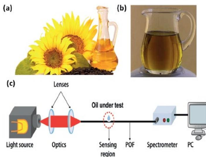
**Figure 1.** (a) Optical photograph of as received sunflower oil (yellow in colour) and (b) exposed sunflower oil (reddish in colour). (c) Absorption/transmission spectrum analyser.
