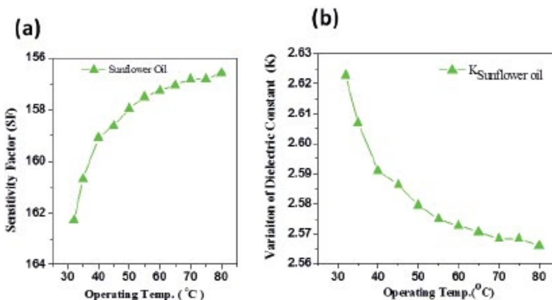
**Figure 4.** Variation of (a) Sensitivity Factor and (b) Dielectric constant ( $k$ ) as function of operating temperature for Sunflower oil.
