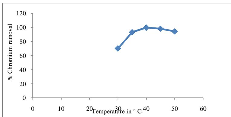
Fig. 5. Effect of Temperature on percentage chromium removal by crude biosorbent
