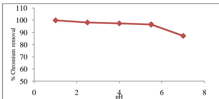
Fig. 2. Effect of pH on percentage chromium by pyrolysed biosorbent
