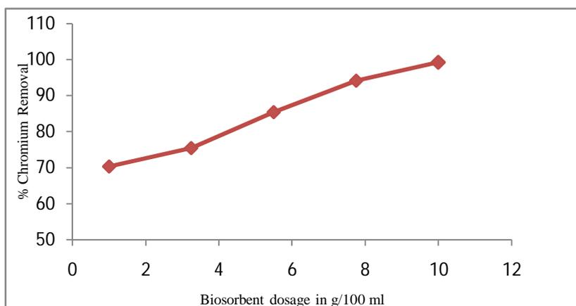
Fig. 8. Effect of pyrolysed biosorbent dosage on percentage chromium removal
