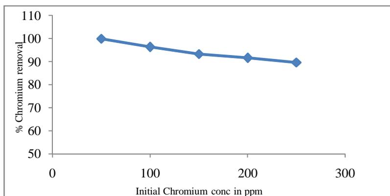
Fig. 3. Effect of initial chromium Concentration on percentage chromium removal by crude biosorbent
