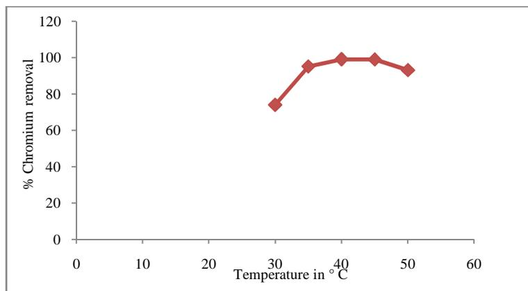
Fig. 6. Effect of Temperature on percentage chromium removal by pyrolysed biosorbent
