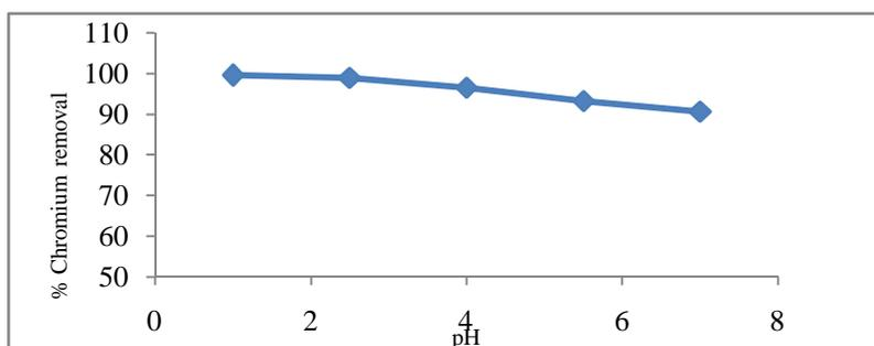
Fig. 1. Effect of pH on percentage chromium removal by crude biosorbent
