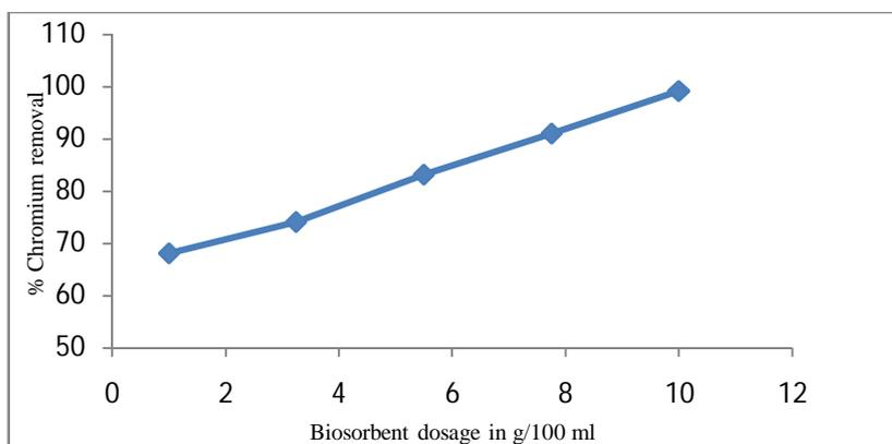
Fig. 7. Effect of crude biosorbent dosage on percentage chromium removal
