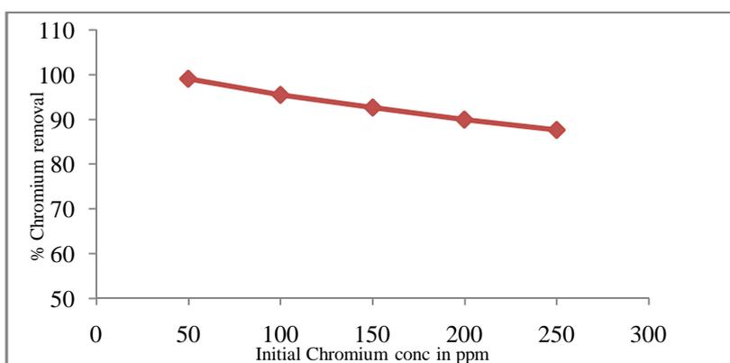
Fig. 4. Effect of Initial Chromium concentration on percentage chromium removal by pyrolysed biosorbent
