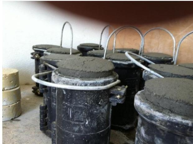
Fig. 3 View of the expansion of concrete samples
