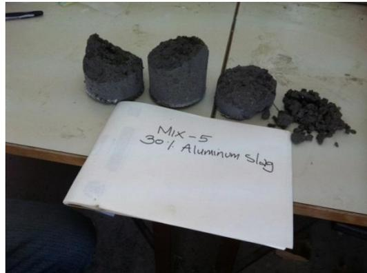
Fig. 4 Broken samples of mixture 5 which contains 30% aluminium dross
