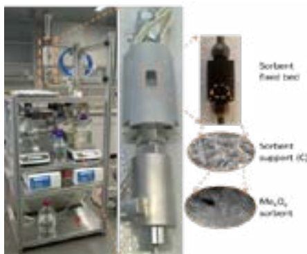
Figure: Dedicated experimental setup for desulfurization under SCW conditions.
