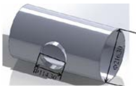
Fig.1 Target shape after burring process
