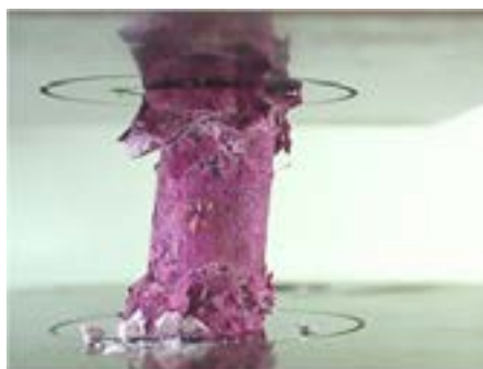
Fig. 1: A sea urchin spine (colored) in compression test displaying the "graceful failure" mechanism
