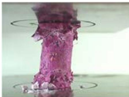
Fig. 1: A sea urchin spine (colored) in compression test displaying the "graceful failure" behavior
