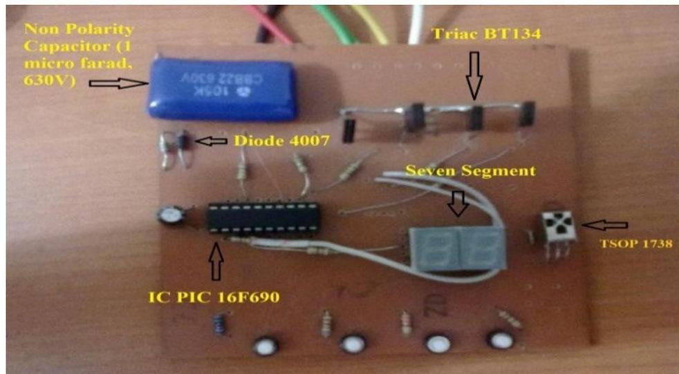
Fig.3: Hardware Implementation of Receiver Circuit
