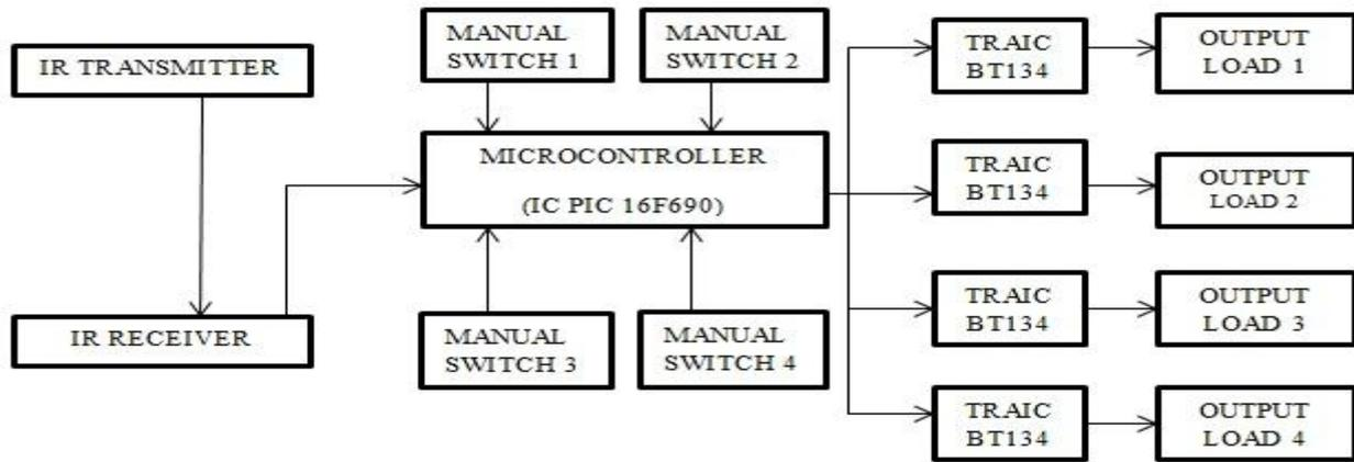
Fig.1: Functional Block Diagram of the System
