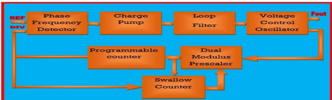
Fig.1 Block diagram of PLL Frequency Synthesizer
