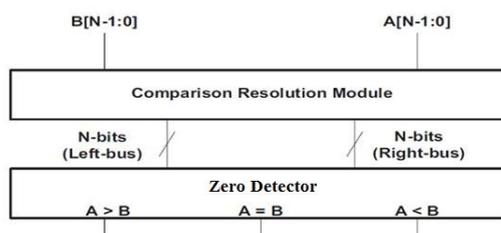
Figure2: Proposed N-Bit-Comparator with Zero Detector as decision module
