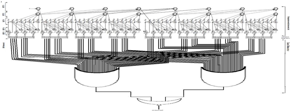
Figure5: The 32-Bit Comparator Using Parallel Prefix Tree Structure with Zero Detector
