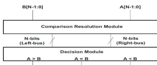
Figure1: Basic Parallel Prefix Tree based N-Bit-Comparator
