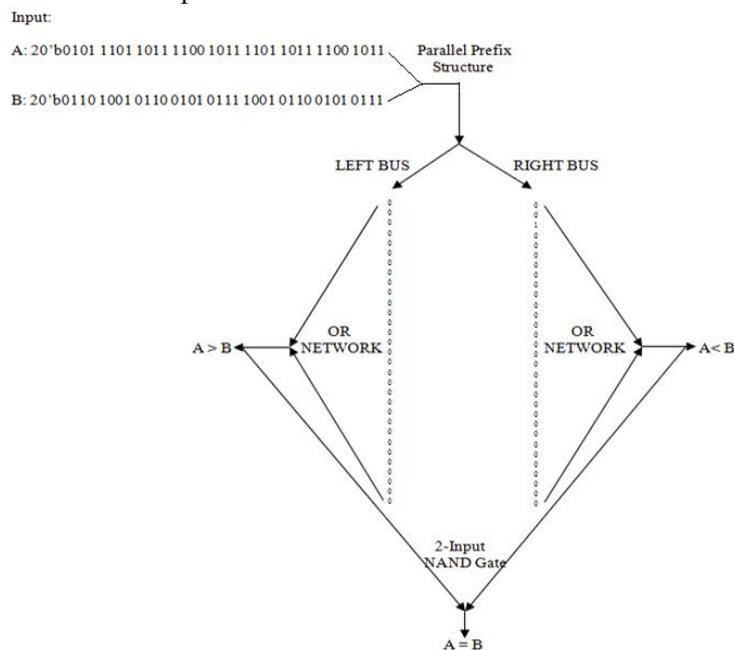
Figure3: Example 32-bit proposed Comparator Architecture
