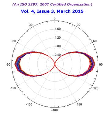
Figure 2: Radiation Pattern of Dipole Antenna (Frequency 0.3 GHz)
