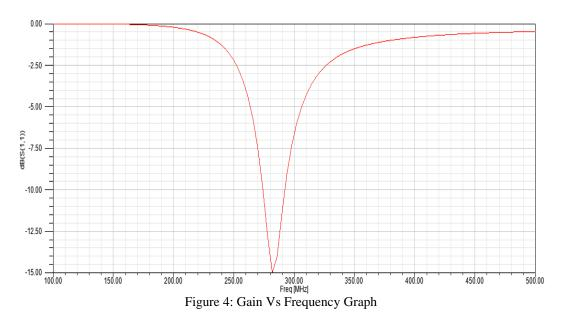
In Figure 4, this figure describe a graph of gain vs frequency.it is clearly shown that when frequency is 160 MHz gain is high but when frequency increasing up to 300 MHz gain is in nadir point after a certain time increase frequency gain also increasing.
