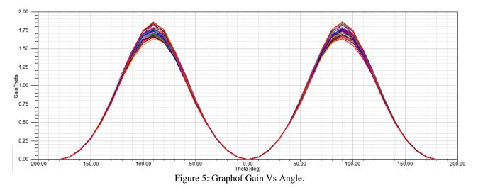
Figure 5 describe graph of gain Vs Angle. Seen that obtain highest gain when the angle is -100 degree or +100 degree. In angle 0 degree gain touch the nadir point. Highest gain obtain from this is around 1.80. After obtained highest gain increasing angle gain will be decreasing.
