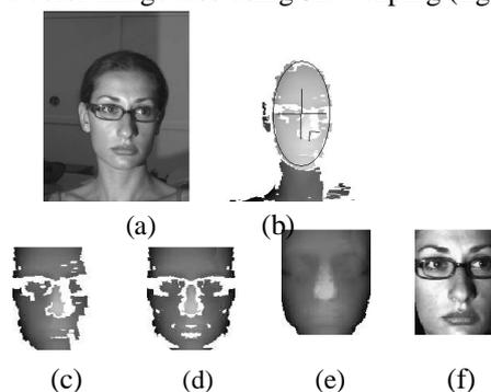
**Fig. 1.** Pose compensation example. (a) Original color image, (b) original depth image showing detected head blob and estimated local coordinate system fixed on the nose, (c) rectified depth image, (d) symmetry-based interpolation, (e) final linear interpolated depth image, (f) rectified color image.
