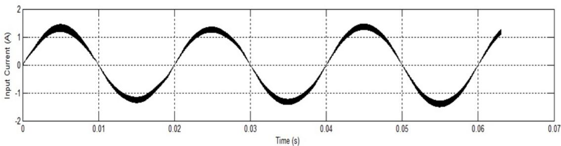
Fig.10 Current waveform at ac mains of Zeta Converter fed BLDC Motor Drive
