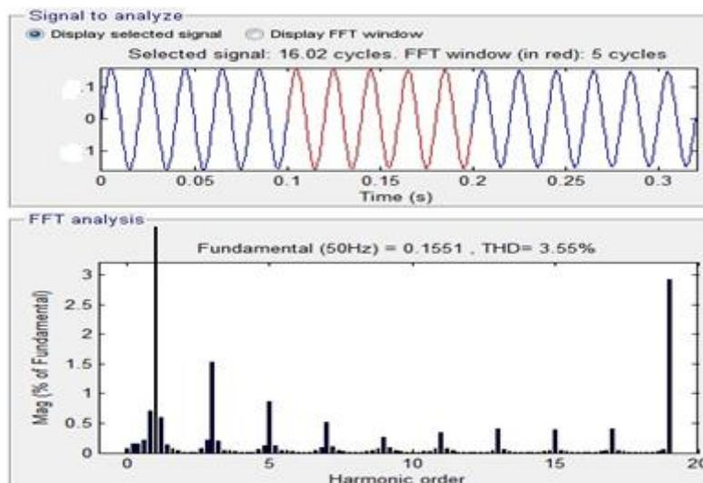
Fig.11 Harmonic Spectra of BLDC Motor Drive with PFC converters
