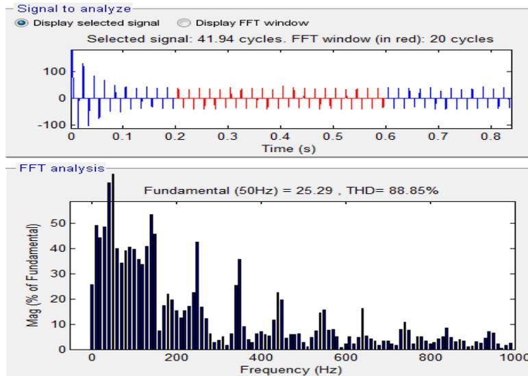
Fig.7 Harmonic Spectra of BLDC Motor Drive without PFC converters
