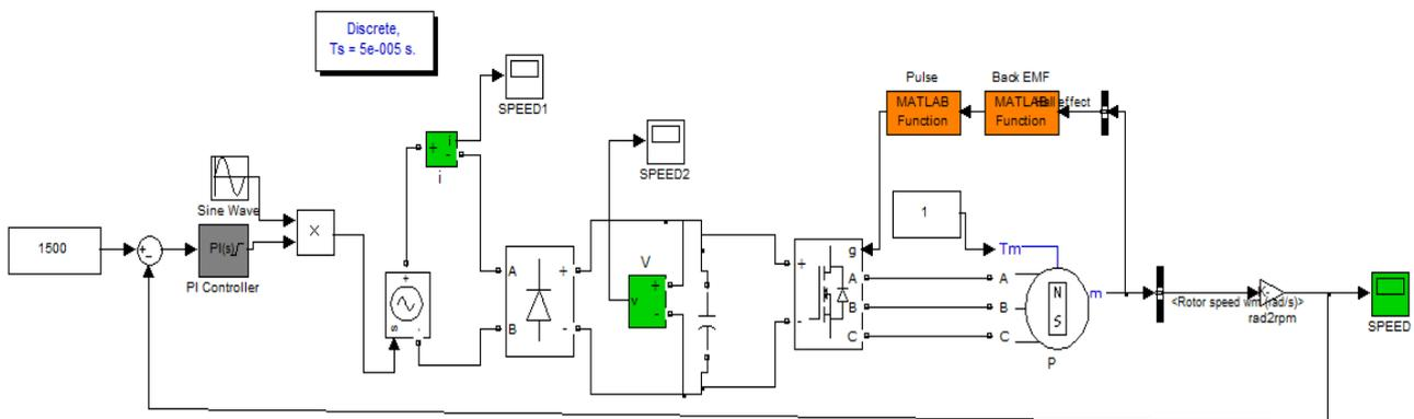
Fig.5 BLDC motor drive without PFC Converter
