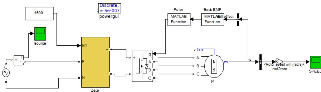
Fig.8 BLDC Motor Drive with Zeta converter for harmonic reduction
