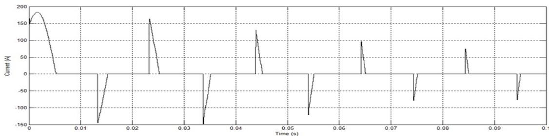
Fig.6 Current waveform at ac mains of BLDCMD without PFC converter
