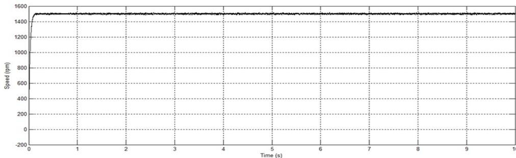
Fig.9 Speed Control of BLDC Motor Drive with Zeta converter
