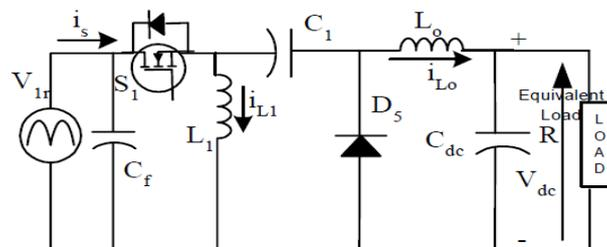
Fig. 1: Circuit of Zeta Converter
