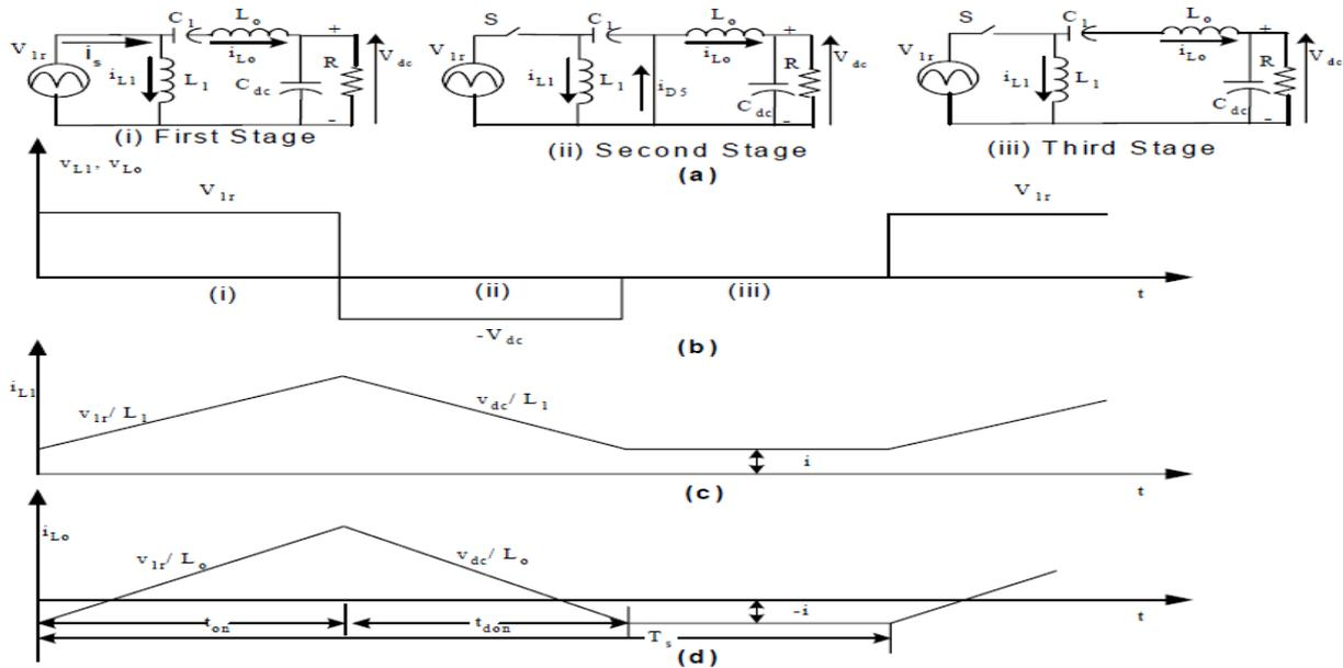
Fig. 2 (a) Three Different Operating Stages (i), (ii) and (iii) of Zeta Converter in DCM of Operation and its (b) Voltage Waveforms (c) and (d) Inductors Current Waveform
