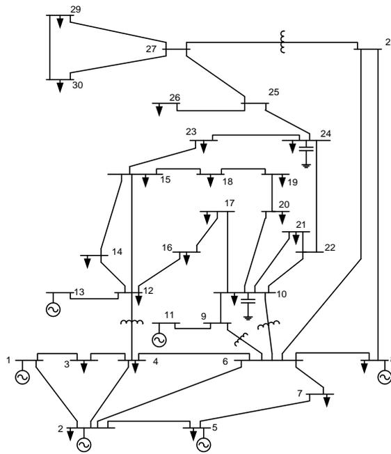
Fig. 1 Single-line diagram of IEEE 30-bus test system [18]
