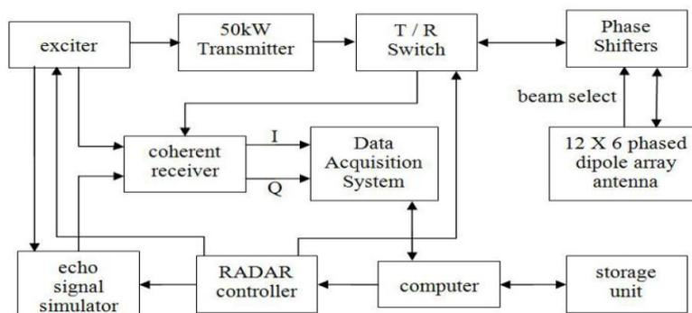
Figure 2. Block Level Architecture of HF Radar
