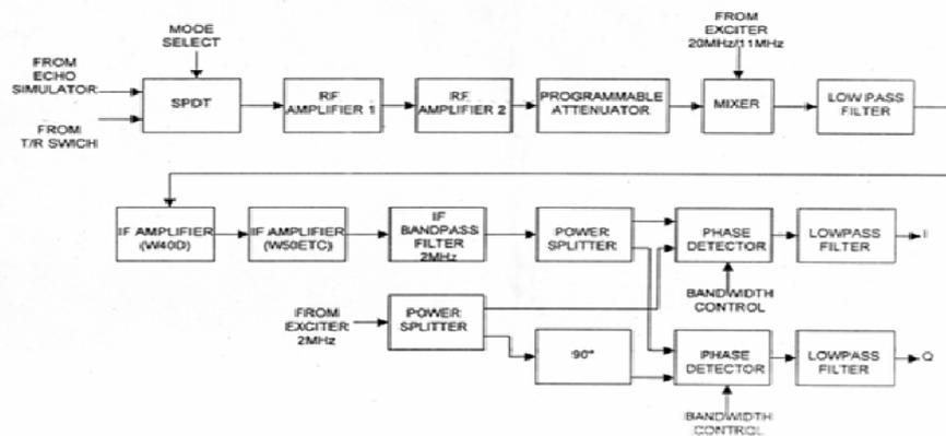
Figure 3. HF receiver Diagram
