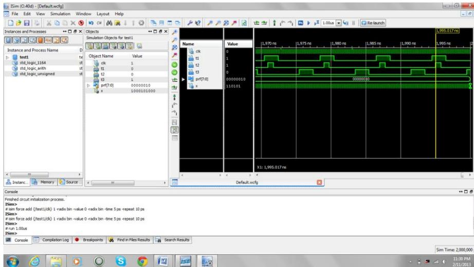
Figure 8. Timing diagram of transmitted RF signal, transmitting pulse, received pulse(at prf =200 and pulse width=80  $\mu$ s)
