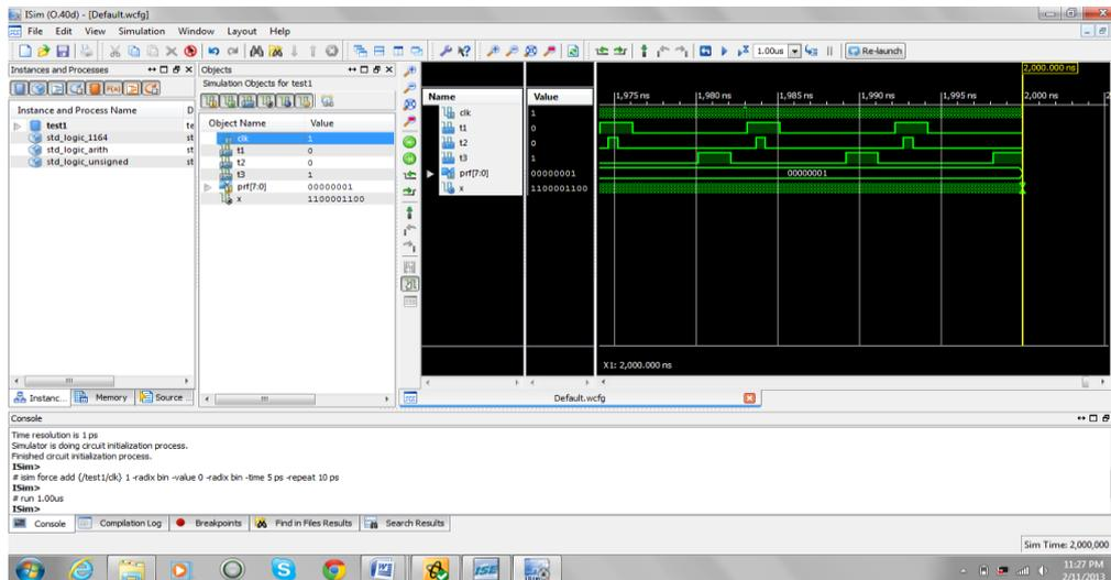
Figure 7. Timing diagram of transmitted RF signal, transmitting pulse, received pulse(at prf =167 and pulse width=60 μs)
