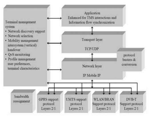
Fig.2 Architecture of a terminal that operates in a composite radio environment
