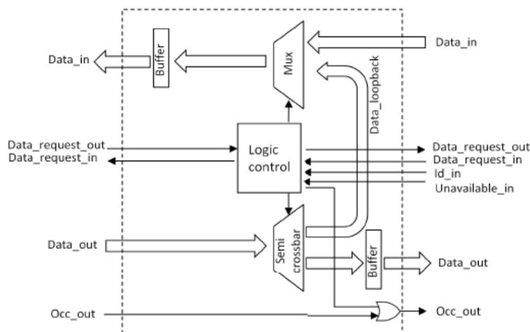
Fig. 3. Architecture of loopback module
