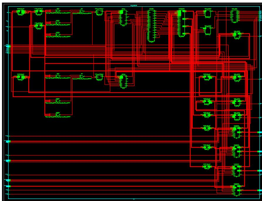
Fig. 8. RTL view of 1×3 mesh using rkt switch
