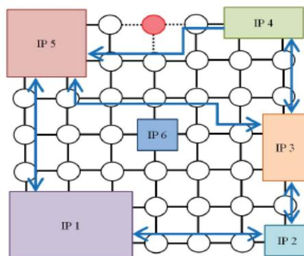
Fig. 1. Bypassing in NoC
