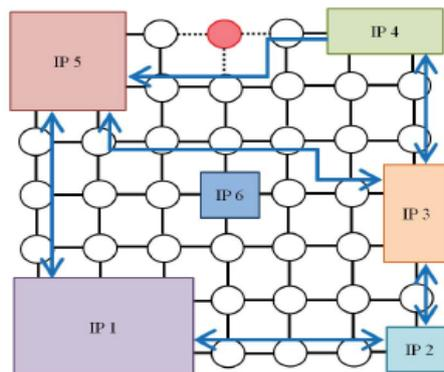
Fig. 1. Bypassing in NoC
