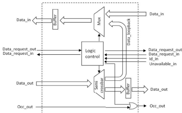
Fig. 3. Architecture of loopback module
