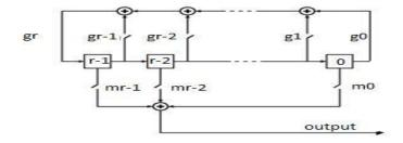
Fig.5 Block diagram of PN sequence
