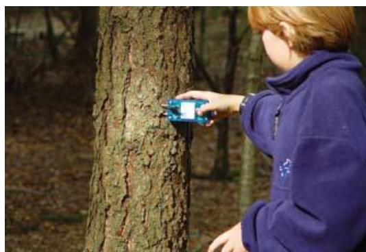
**Fig-6** Ubi-learning in the Ambient Wood (University of Sussex):a boy using a digitally augmented probe tool that shows real time measurements of light and moisture on an accompanying mobile device
