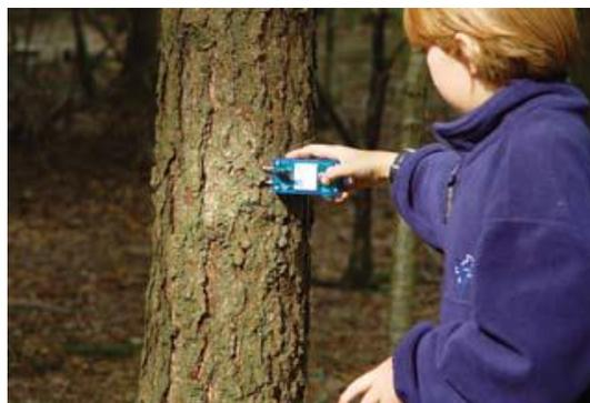
**Fig-6** Ubi-learning in the Ambient Wood (University of Sussex): a boy using a digitally augmented probe tool that shows real time measurements of light and moisture on an accompanying mobile device
