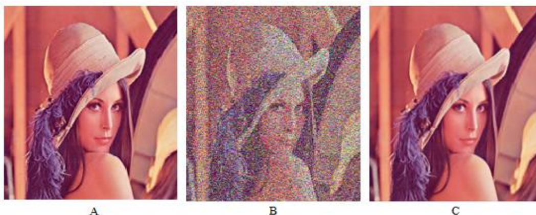
Fig. 2: A. origin image. B. noisy image with salt & pepper noise. C. image after de-noising using STLS.
