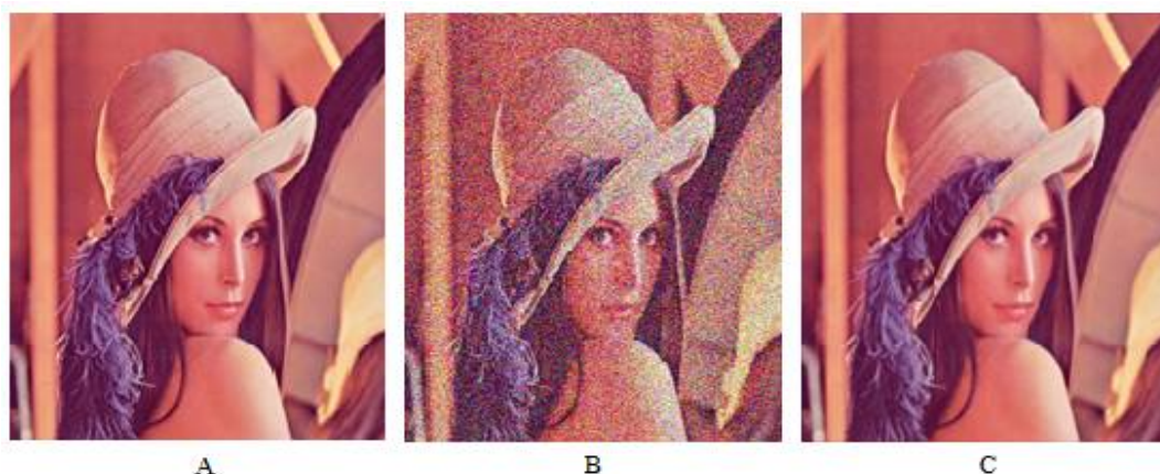
Fig. 3: A. origin image. B. noisy image with Gaussian noise. C. image after de-noising using STLS.
