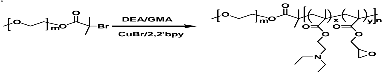
Scheme 1. Schematic illustration for preparation of PEO-b-P(DEA-co-GMA).
