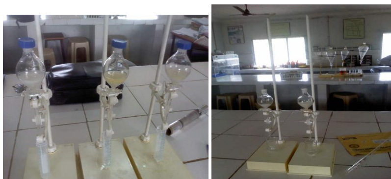
Figure 2: A. filling of column by silica gel. B. Separation of antibiotic by column chromatography.
