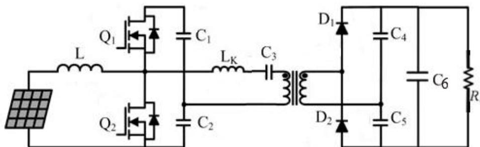
Fig 3. Integrated Boost Series LC Resonant Converter
