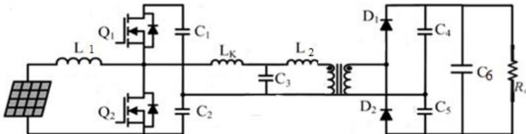
Fig 5. Integrated Boost LLC Resonant Converter
