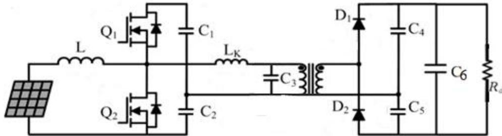
Fig 4. Integrated Boost Parallel LC Resonant Converter
