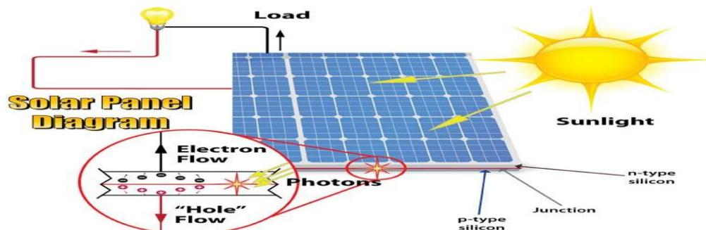
Fig 2 Production of electricity from Solar PV Panel
