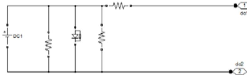
Fig .8 Solar PV Equivalent Circuit
