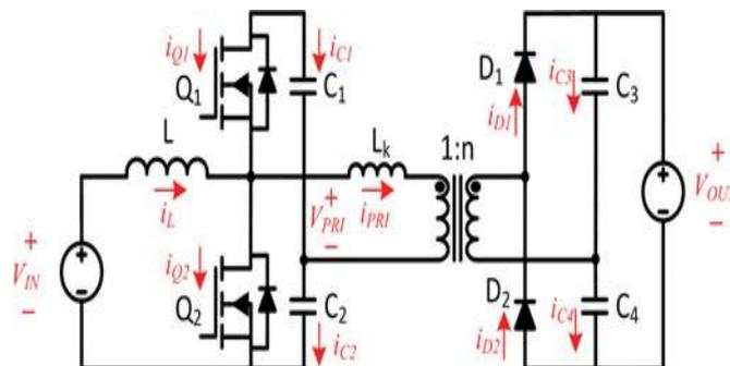
Fig 1. An Integrated Boost Resonant Converter
