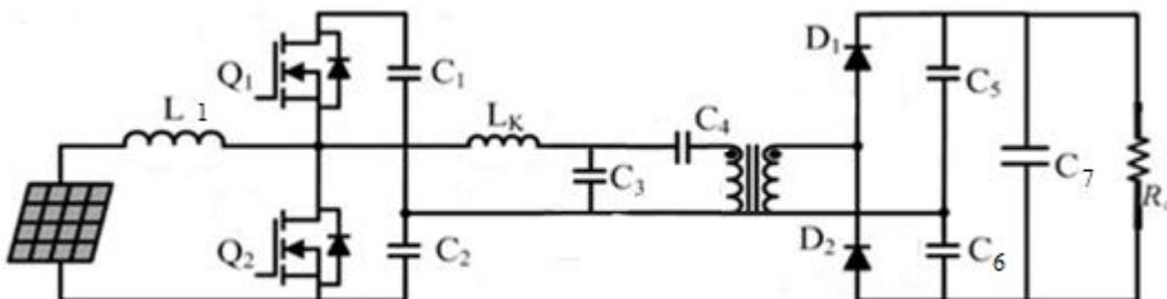
Fig 6. Integrated Boost Series LC Resonant Converter
