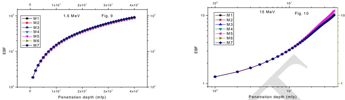
Fig. 7-10 Variation of Exposure buildup factor of selected samples with penetration depth up to 40 mfp at 0.015MeV, 0.15 MeV, 1.5 MeV and 15MeV
