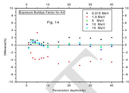
Fig. 14 Difference(%) between ANSI data and our work with respect to the calculated values of EBF for air at some energy levels upto 40 mfp
