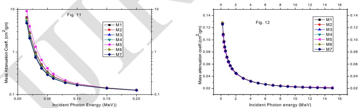
Fig. 11-12 Variation of mass attenuation coefficients with incident photon energy range of 0.015-0.20 MeV and 0.2-15 MeV
