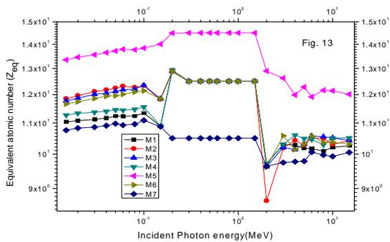
Fig. 13 Variation of equivalent atomic numbers with incident photon energy range of 0.015-15 MeV
