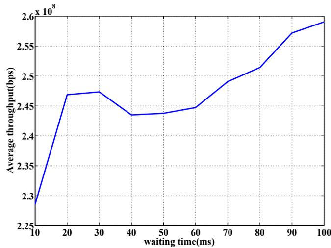
Fig. 6: Throughput Vs. waiting time at packet size = 80,000 Bytes
