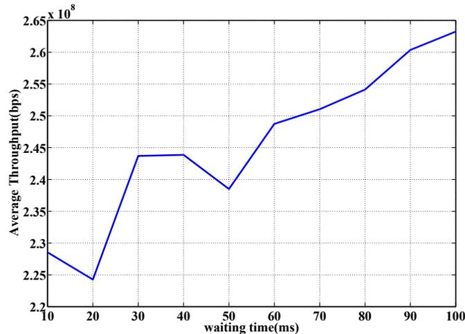
Fig. 7: Throughput Vs. waiting time at packet size = 1,00,000 Bytes
