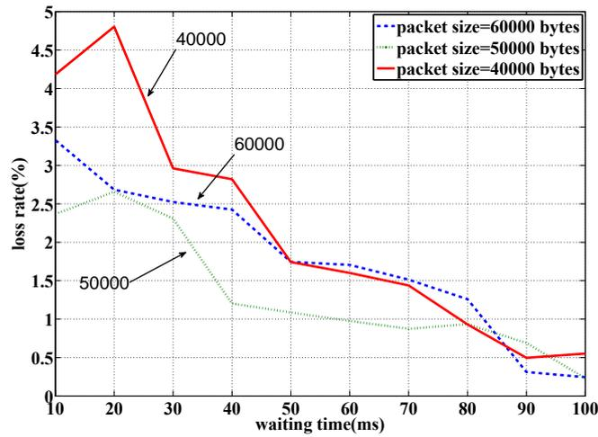
Fig. 3: Waiting time Vs. Loss rate for simple network
