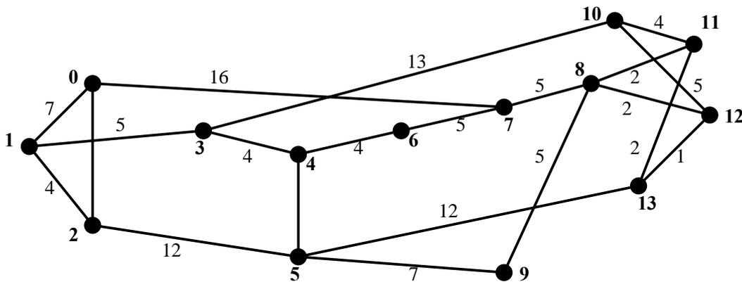
Fig. 2: 14-node NSFNET network with propagation delays
