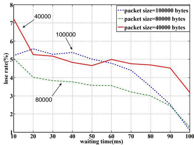
Fig. 4: Waiting time Vs. Loss rate for NSFNET network
