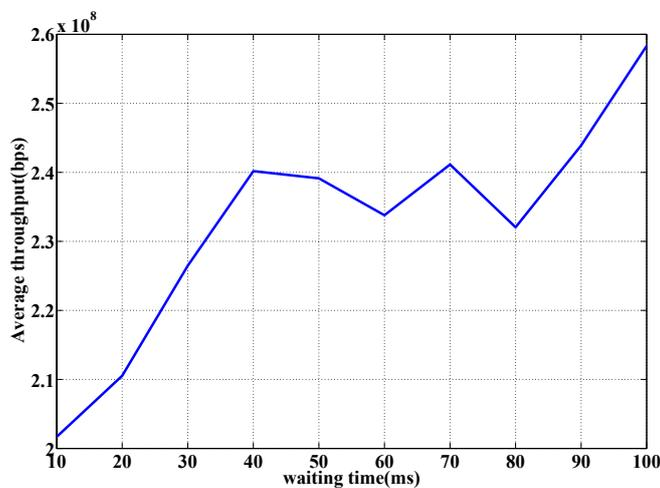
Fig. 5: Throughput Vs. waiting time at packet size = 60,000 Bytes
