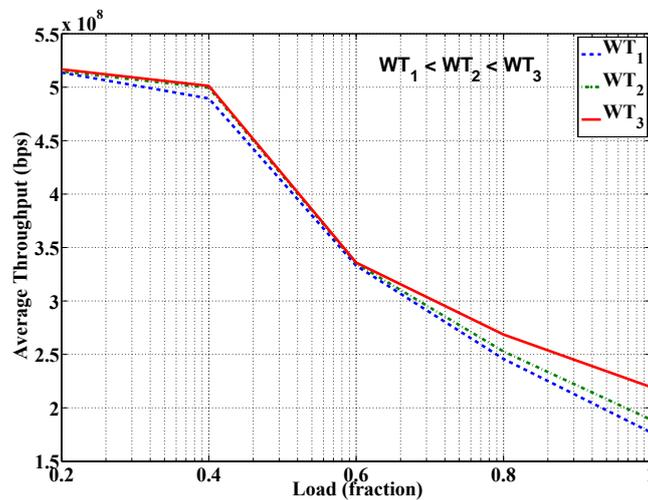
Fig. 9: Throughput Vs. Load at packet size = 80,000 Bytes
