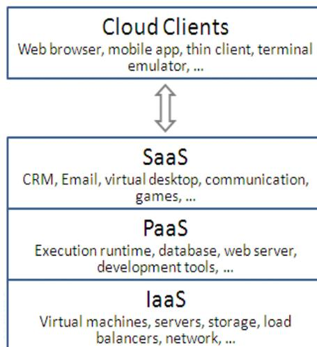
Fig.2. Layers of Cloud Computing.
