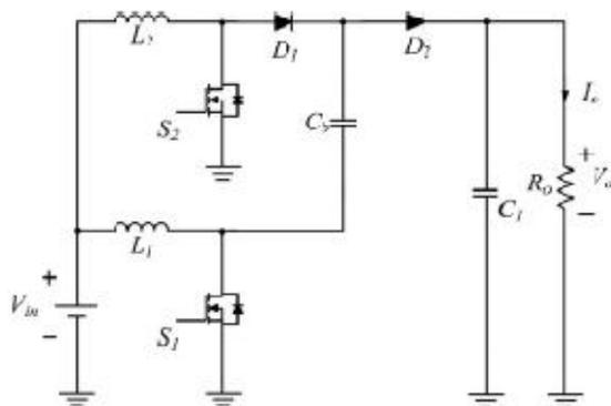
Fig.1. Interleaved boost converter with a voltage-lift capacitor structure.
