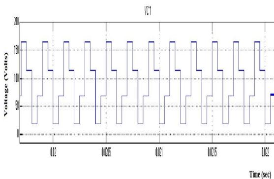
Fig. 6. Output filter capacitor (C1) voltage.
