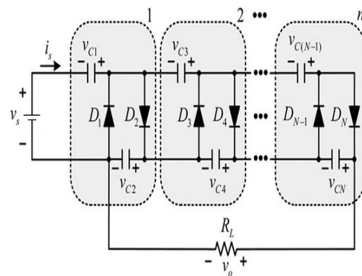
Fig. 4. Conventional n-stage CW voltage multiplier.
