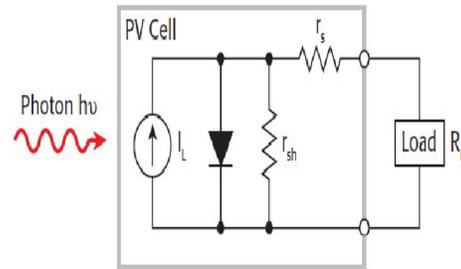
Fig. 3. Equivalent circuit of photovoltaic module.
