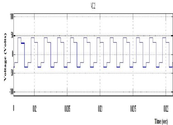
Fig. 7.Output filter capacitor (C2) voltage.
