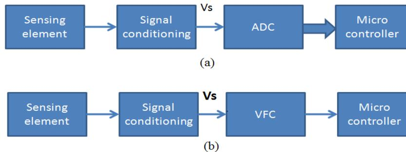
Fig.1.1 (a) Conventional sensing system using ADC and (b) Sensing system using V/F converter
