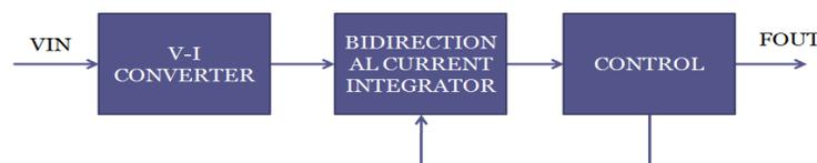
Fig.2.1 Multivibrator based VFC architecture
