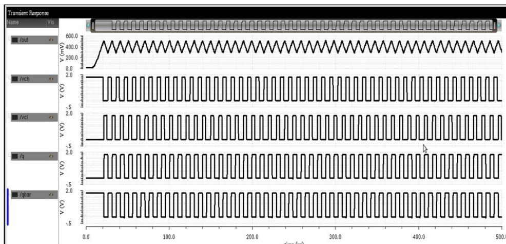
Fig.3.1 Intermediate and output waveforms of the proposed VFC
