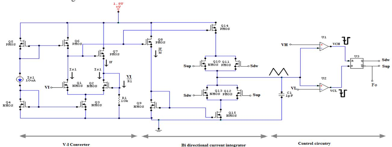
Fig.2.2 Complete schematic diagram of the CMOS multivibrator based VFC
