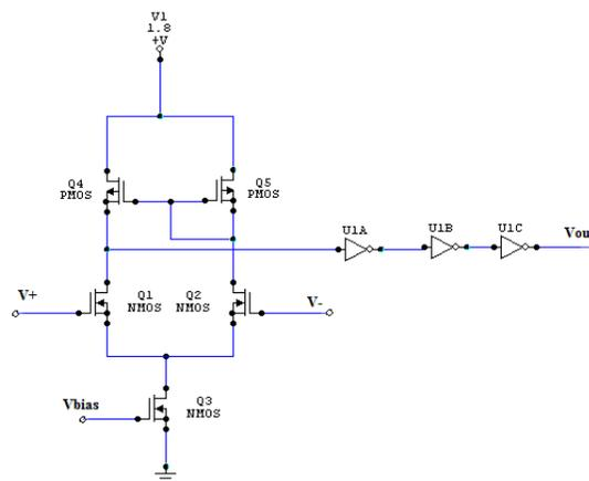
Fig.2.3 (a) Complete schematic diagram of the CMOS multivibrator based VFC
