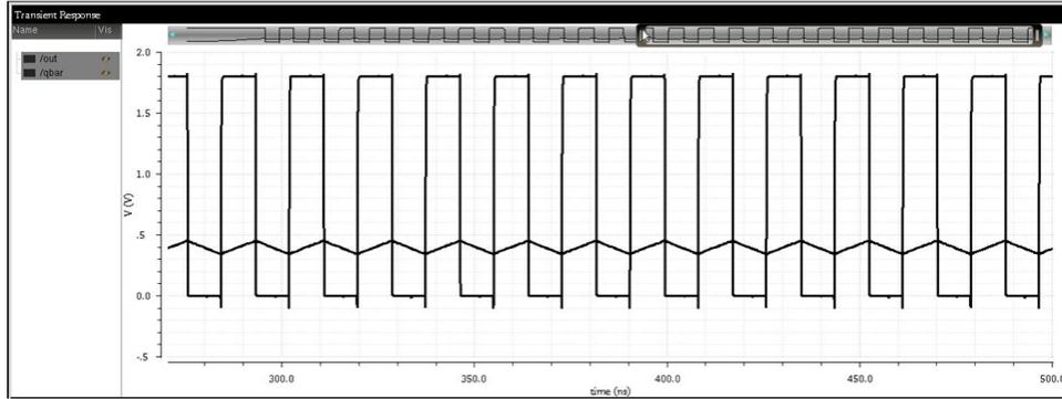
Fig.3.3 Vcap and FO for  $V_I=0.6V$
