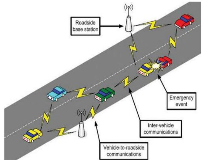
Figure 1.3 Schematic Representation of a Vehicular Adhoc Network
