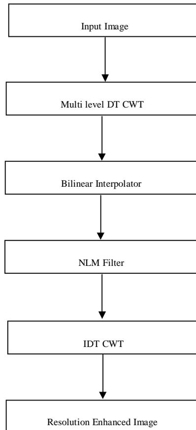
Fig 2 Process Flow Diagram of the Proposed System.
