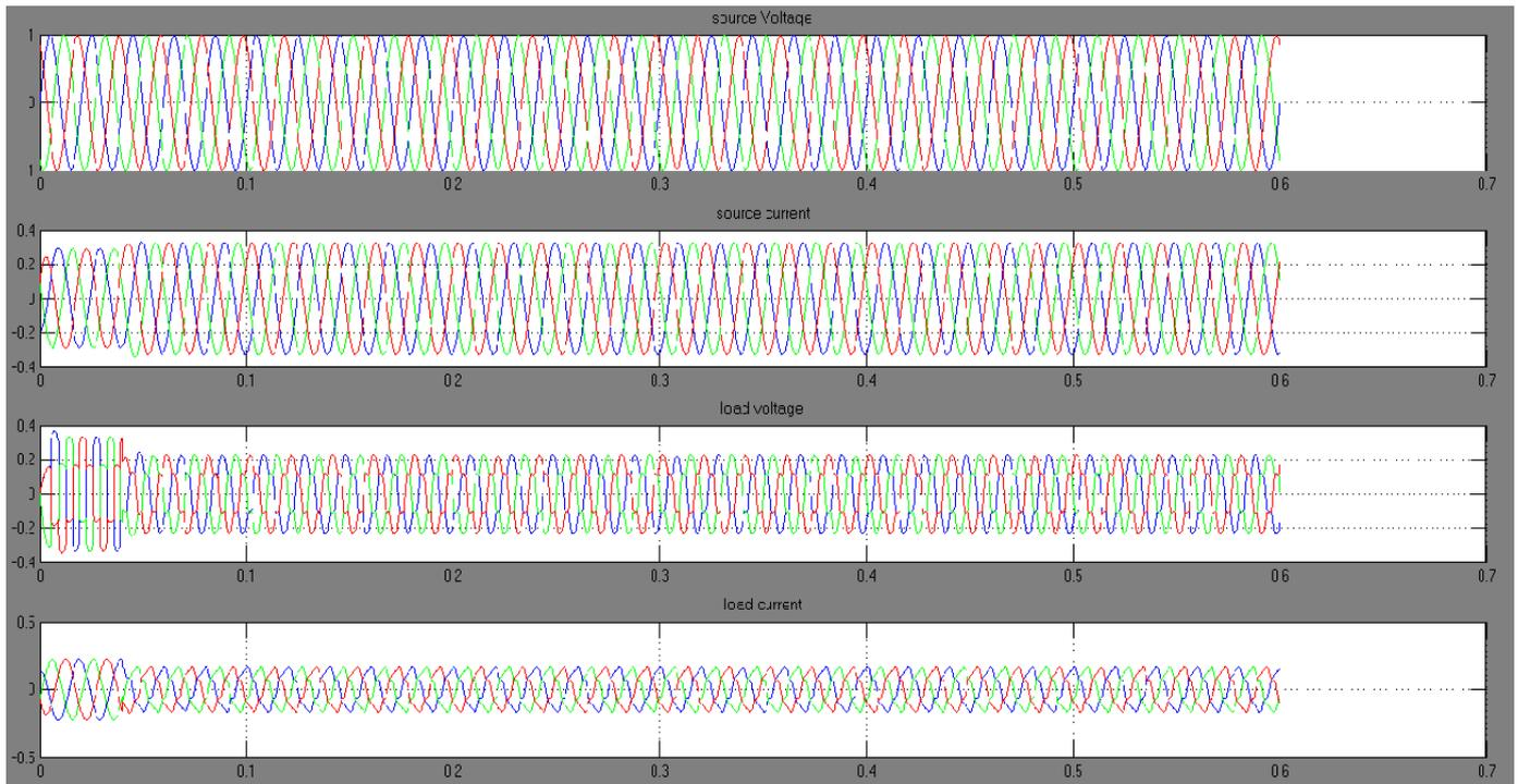
Fig.2. Simulated Voltage and Current Waveform at 50MW 0.8pf. without Transformers core Saturation.
