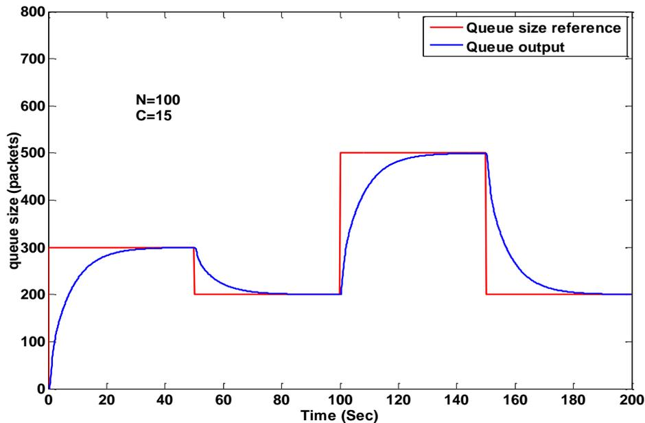
Figure 11: The Queue Length Response with the MR. Wavelet PID Controller for NUM=5,db=6 and N=100
