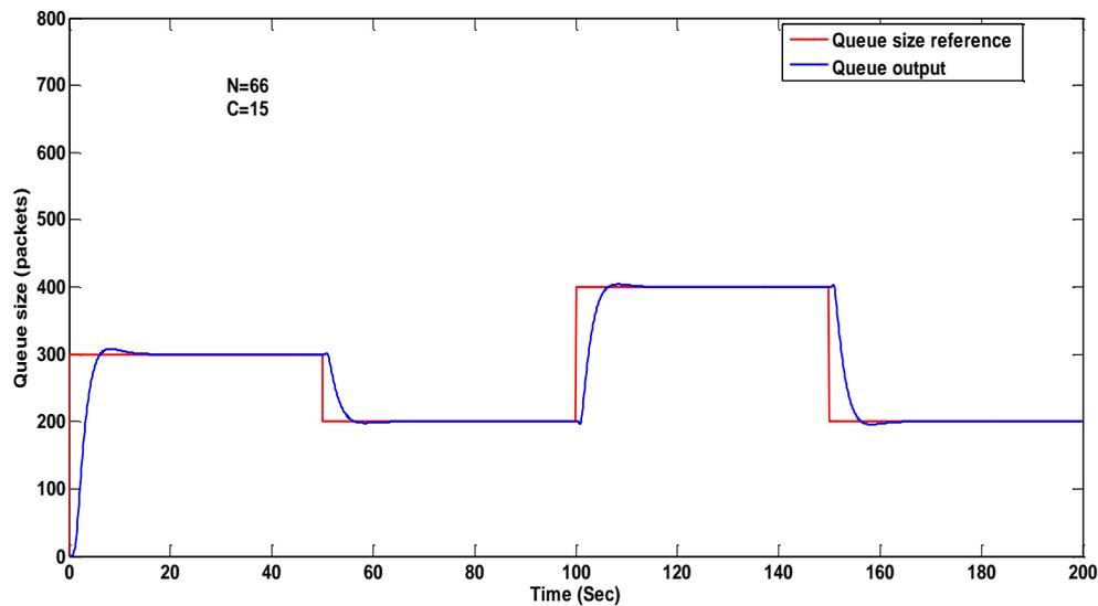
Figure 8: System Response with db 2 and NUM=3 with (N=66 nodes) of TCP Flows.
