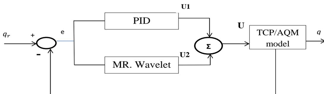
Figure 2: Hybrid of PID with MR. Wavelet
