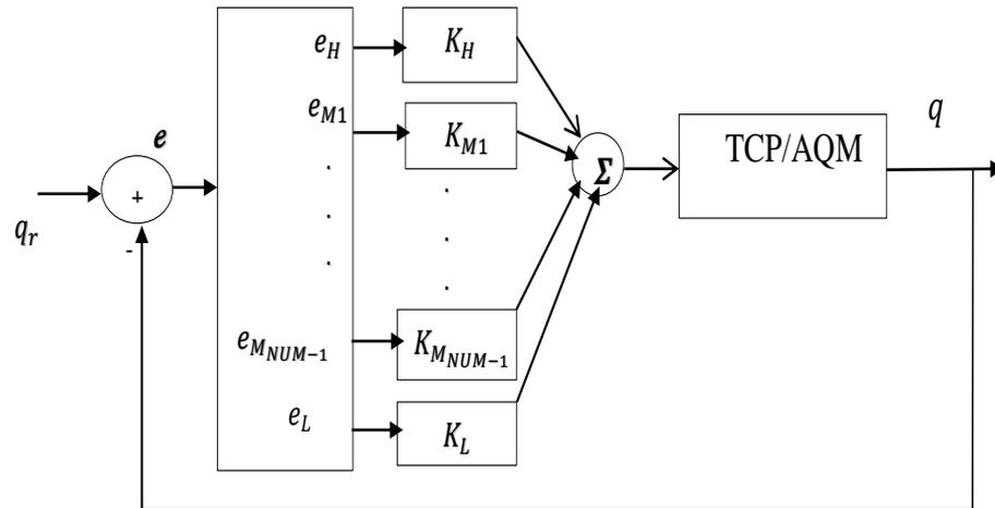
Figure 1: Block diagram of MR. Wavelet
