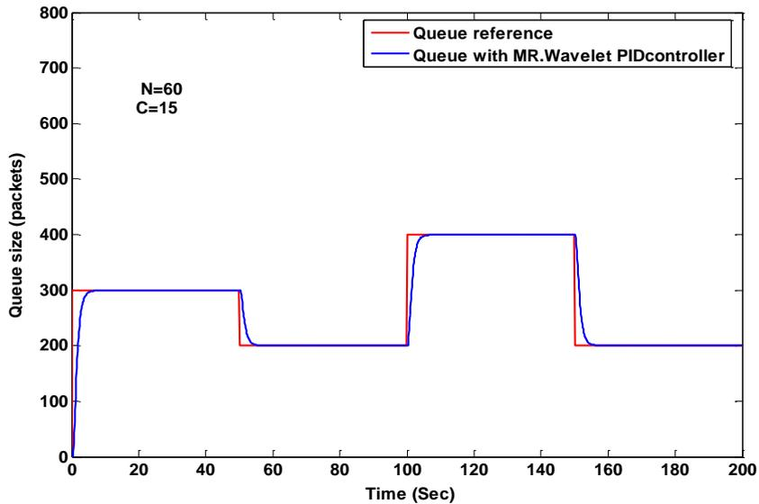
Wavelet PID with NUM=3 and db2 and the classical PID controllers. The overall performance characteristics for the three controllers are summarized by table (1).
