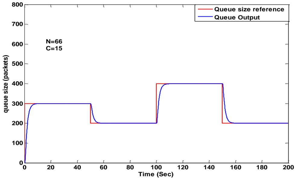
Figure 9: System Response with db 6 and NUM=5 with (N=66 nodes)of TCP Flows
