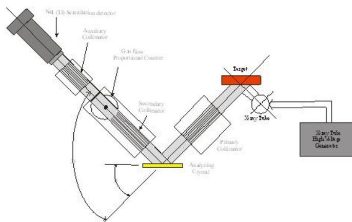
**Figure 2:** Schematic diagram of WDXRF setup.
