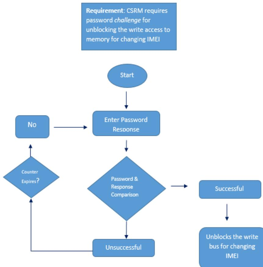
Figure 5: Flow chart for Password challenge and Response mechanism for changing IMEI.
