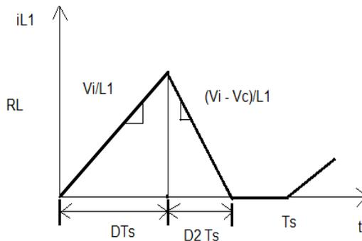
Fig.3 DCM Inductor Current
