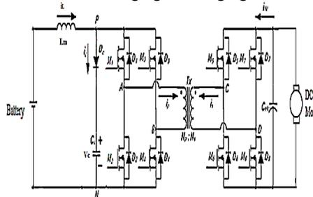
Fig.1 Bidirectional DC-DC Converter
