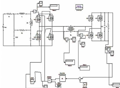
Fig.5 Simulation circuit of bidirectional full bridge DC-DC converter with RCD snubber
