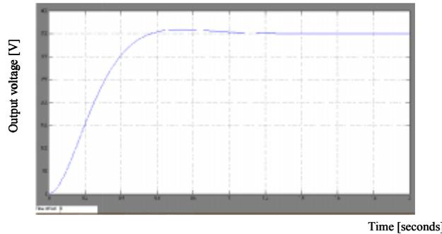
Fig.13 Simulation result of bidirectional full bridge DC-DC converter with flyback snubber with DC Motor - Boost open loop operation with output voltage 350V.
