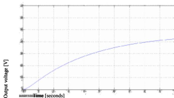
Fig.18 Simulation result of open loop bidirectional full bridge DC-DC converter without flyback snubber- Buck operation
