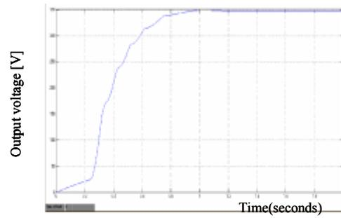
Fig.6 Simulation result of bidirectional full bridge DC-DC converter with RCD snubber
