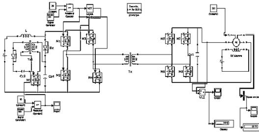
Fig.11 Simulation circuit of bidirectional full bridge DC-DC converter with flyback snubber with DC Motor - Boost open loop operation
