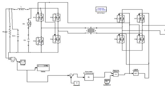
Fig.21 Simulation circuit of bidirectional full bridge DC-DC converter with flyback snubber with DC Motor – Buck closed loop operation
