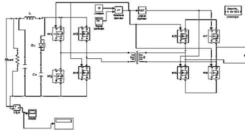
Fig.19 Simulation circuit of bidirectional full bridge DC-DC converter with flyback snubber with DC motor- Buck open loop operation
