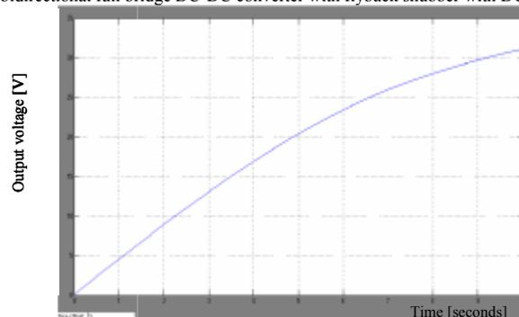
Fig.22 Simulation result of bidirectional full bridge DC-DC converter with flyback snubber with DC Motor – Buck closed loop operation with an output voltage of 32.5V
