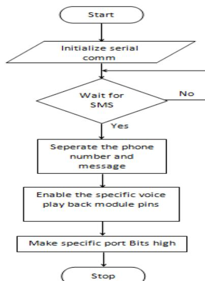
Fig 2: Flow diagram of sender side part 1
