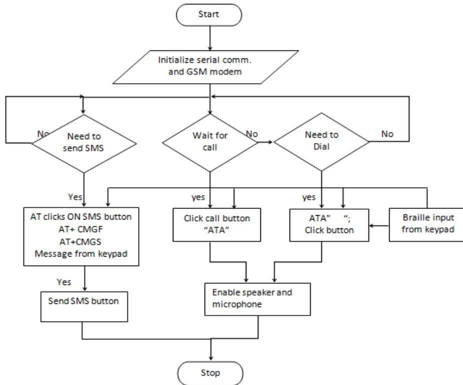
Fig 3: Flow diagram of sender side part2
