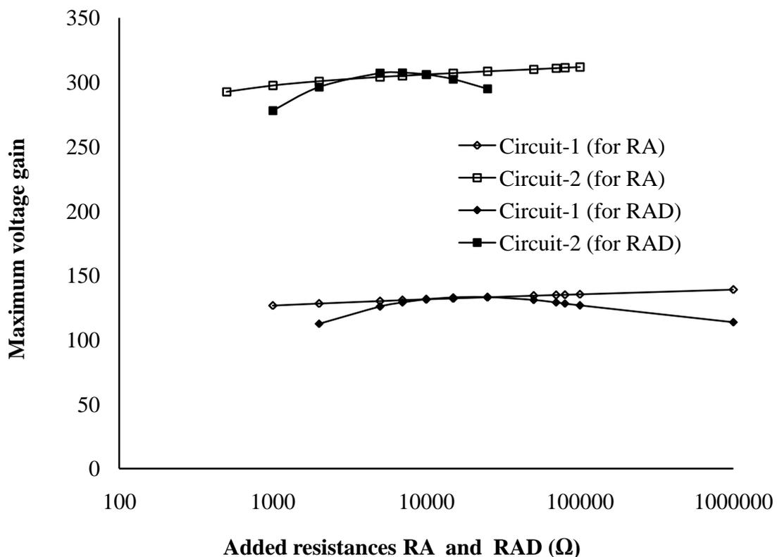
Fig.5. Variation of Maximum voltage gain with  $R_A$  and  $R_{AD}$
