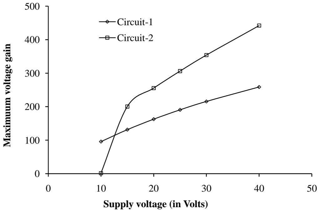
Fig.2. Variation of Maximum voltage gain with  $V_{CC}$
