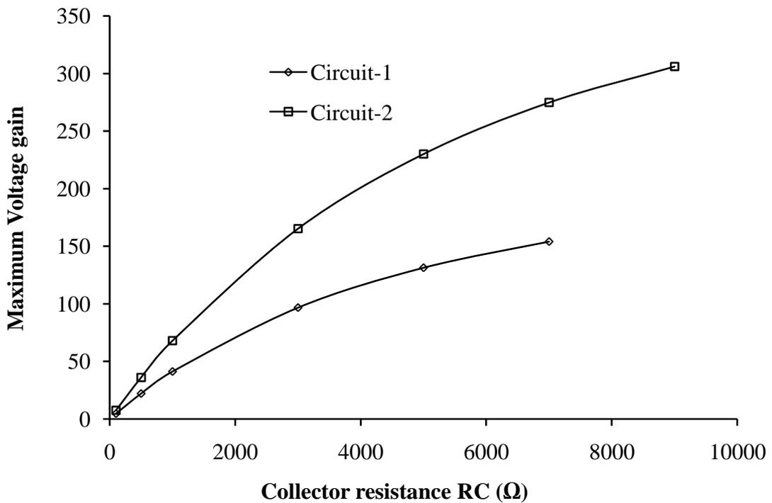
Fig.4. Variation of Maximum voltage gain with  $R_C$
