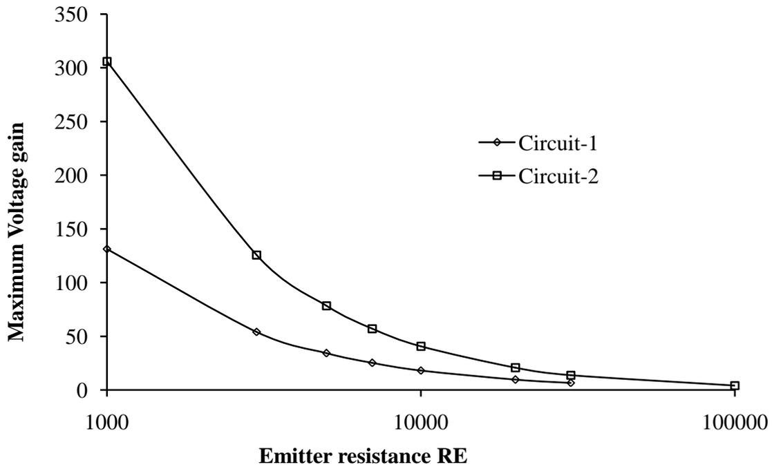
Fig.3. Variation of Maximum voltage gain with  $R_E$
