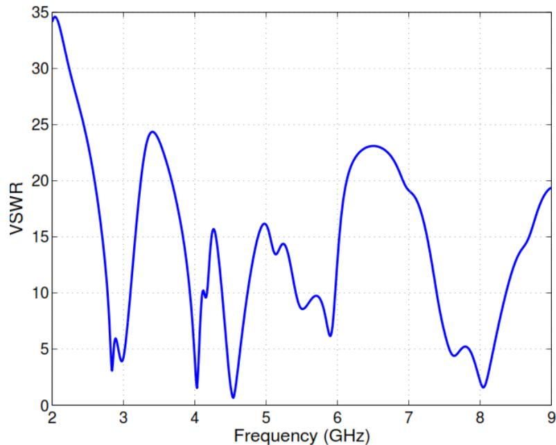
**Figure 5: VSWR of proposed antenna design.**
