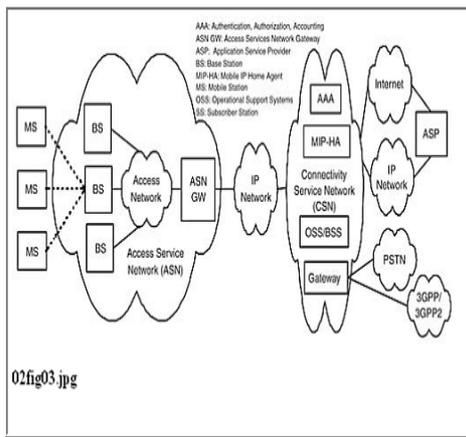
Fig. 1 System Model and Problem Specification
