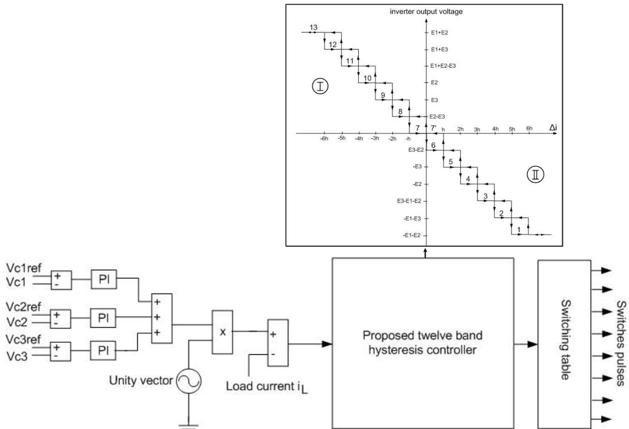
Figure 3.the proposed balancing technique of the proposed inverter
