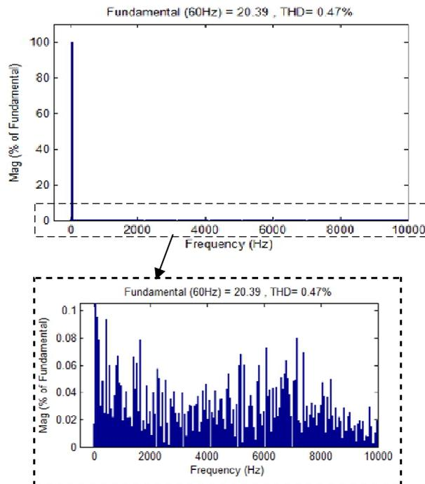
Figure 7. Harmonics spectrum of load current with loop effect
