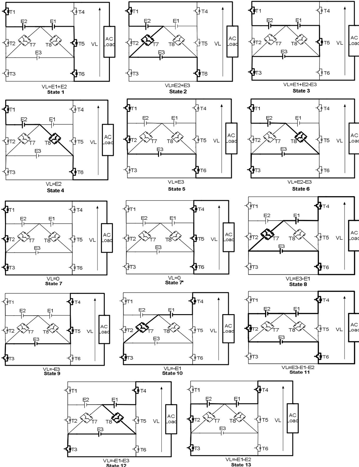
Figure 2. One cycle operating states of the proposed inverter
