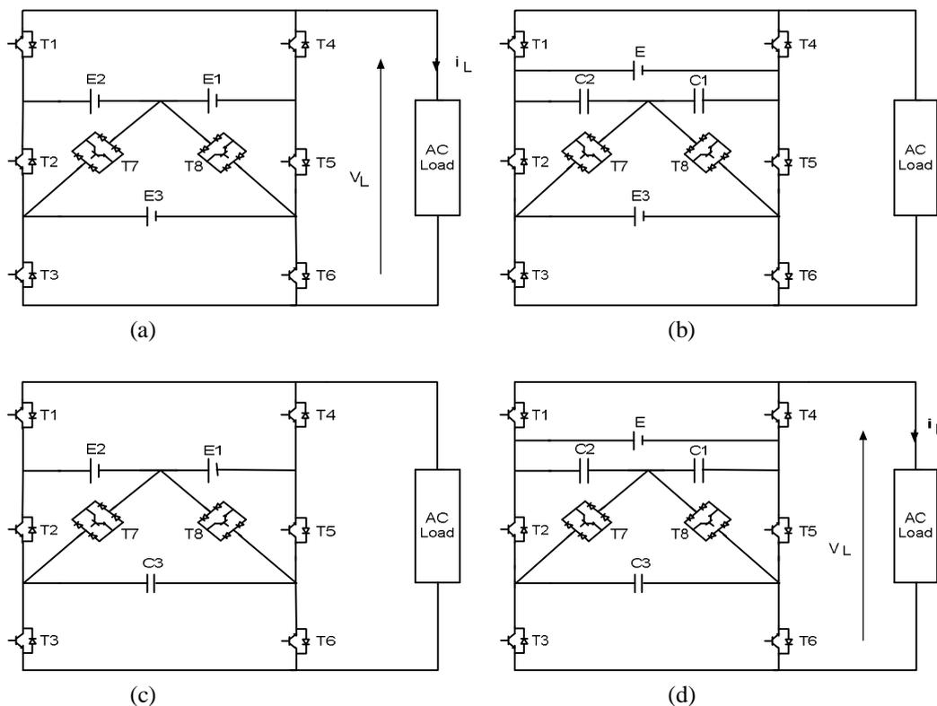
Figure 1. The proposed multilevel inverter with: (a) three DC sources required (b) two DC sources and two capacitors required (c) two DC sources and one capacitor required (d) one DC source and three capacitors required
