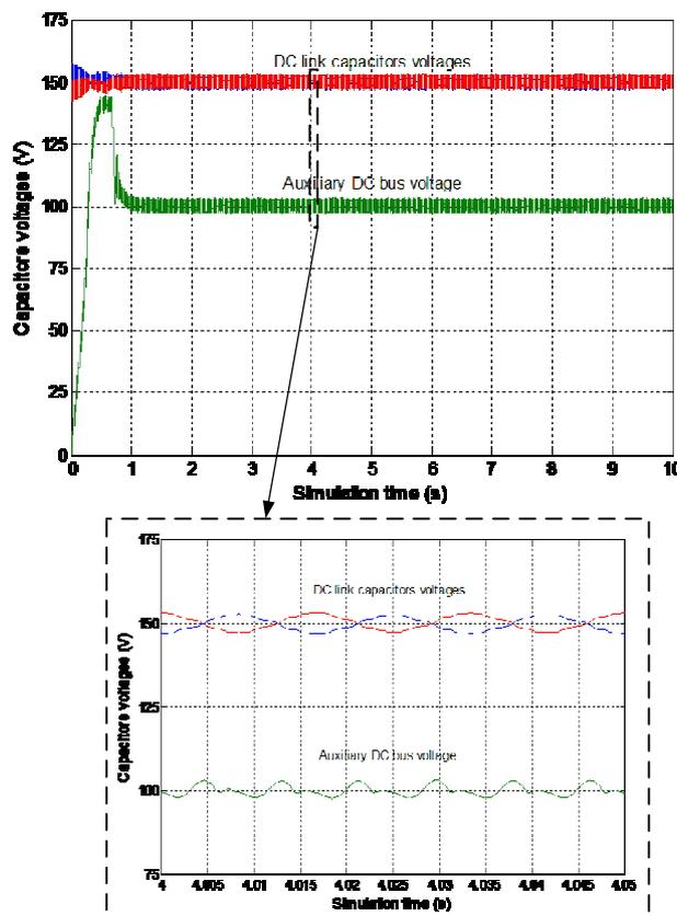
Figure 4. Capacitors voltages evolution
