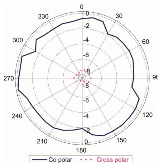
Fig. 5 Typical radiation pattern of HCRMA measured at 7.45 GHz
