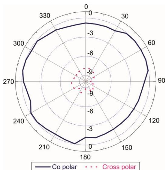
Fig. 6 Typical radiation pattern MHCMA measured at 7.41 GHz
