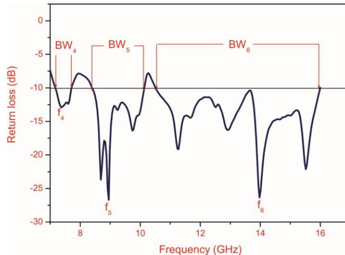
Fig. 4 Variation of return loss versus frequency of MHCMA
