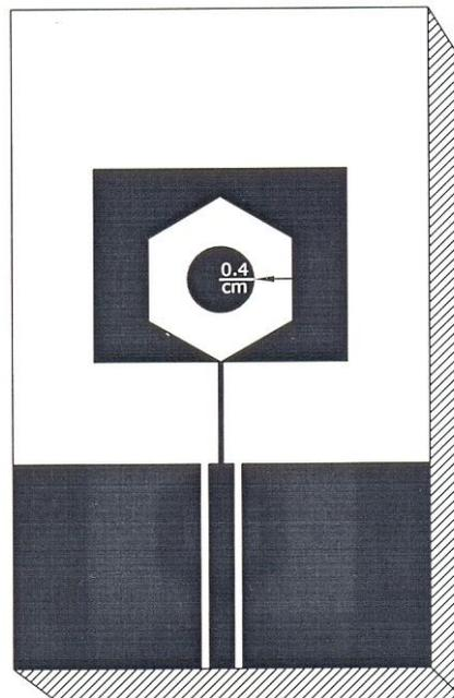
Fig. 2 Top view geometry of MHCRCMA
