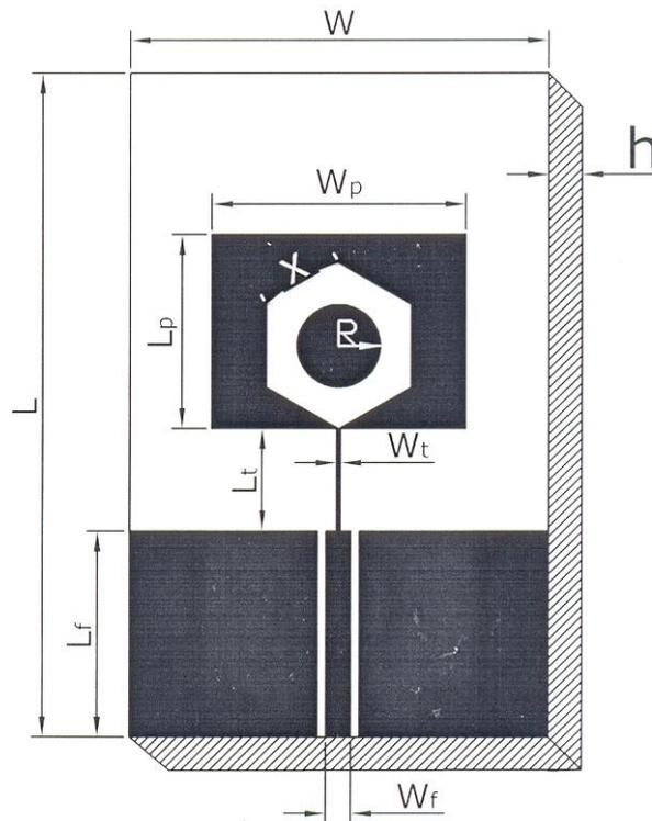
Fig. 1 Top view geometry of HCRMA
