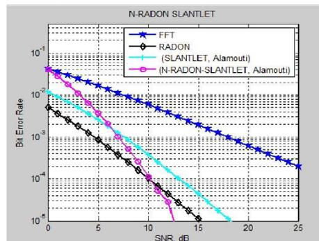
Figure 6: BER performance of RAT-SLT-OFDM in FFC at Doppler frequency 4Hz
