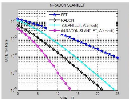
Figure 5: BER performance of NRAT-SLT-based OFDM in AWGN channel.
