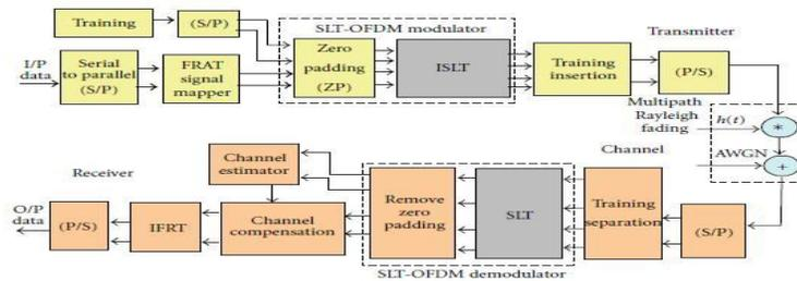
Figure :4 N-Radon-Slt-Based Ofdm Transceiver
