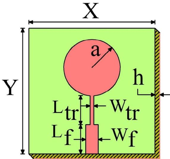
Fig. 1 Top view configuration of CCMSA
