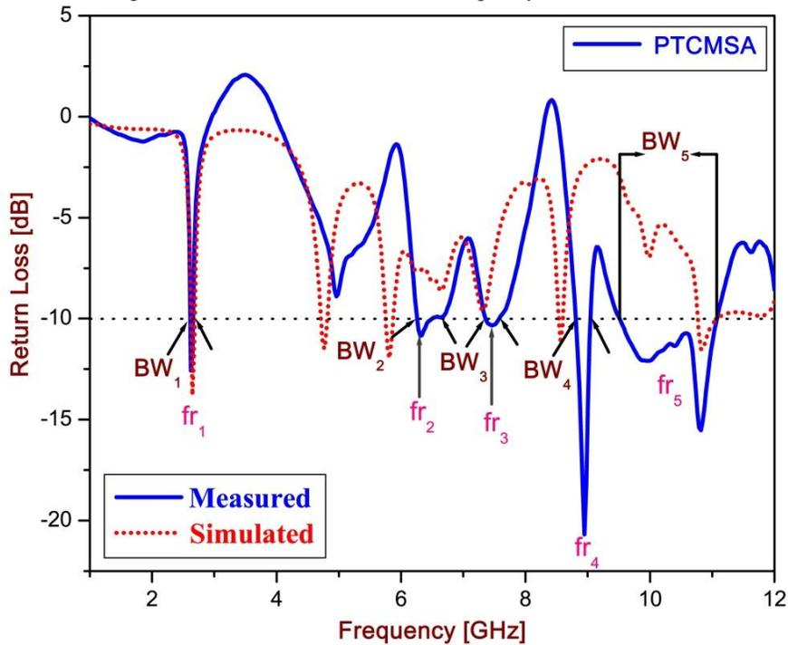
Fig. 4 Variation of return loss versus frequency of PTCMSA
